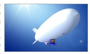
station and operational cost advantages when delivering 360° perspective of the air and ground environment, Aeros' long-loitering 40E airship features useful payload greater than one ton, and supports ISR mission success and efficiency with multi-payload mounting systems for radar, EO/IR cameras, remote sensing technology (LIDAR), and/or
