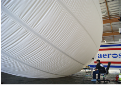
Pressure testing the 40E aft ballonnet following assembly
