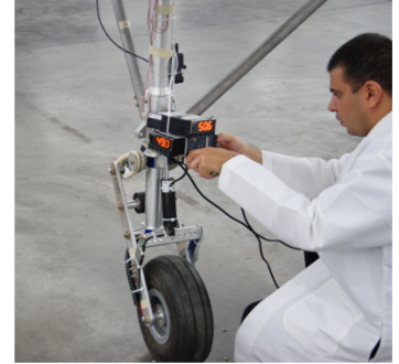
Testing of new landing gear providing pilots static lift data
